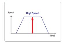
The Ezi-SERVO<sup>®</sup> functions well at high speed without the loss of Synchronism or positioning error. Ezi-SERVO's ability of continuous monitoring of current position enables the stepping motor to generate high-torque, even under a 100% load condition.
