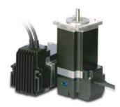
High speed, high precision drive and stepping motor integrated into one package, Ezi-STEP® is unique as it adopts a new control scheme based on a built in high performance DSP(Digital Signal Processor) and software. Ezi-STEP® utilizes a unique position estimation algorithm which instantaneously detects out of synchronization of the stepping motor rotor, which is not available with conventional stepping motor & drives.
