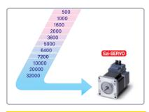
The unit of the position command can be divided precisely. (Max. 32,000 pulses/revolution)
