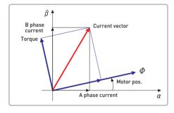
Ezi-SERVO®is a high-precision servo drive, using a high-resolution encoder with 32,000 pulses/revolution. Unlike a conventional Microstep drive, the on-board high performance DSP (Digital Signal Processor) performs vector control and filtering, producing a smooth rotational control with minimum ripples.
