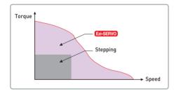
Compared with common step motors and drives, Ezi-SERVO® motion control systems can maintain a high torque state over relatively long period of time. This means that Ezi-SERVO continuously operates without loss of position under 100% of the load. Unlike conventional microstep drives, Ezi-SERVO® exploits continuous high-torque operation during high-speed motion due to its innovative optimum current phase control.
