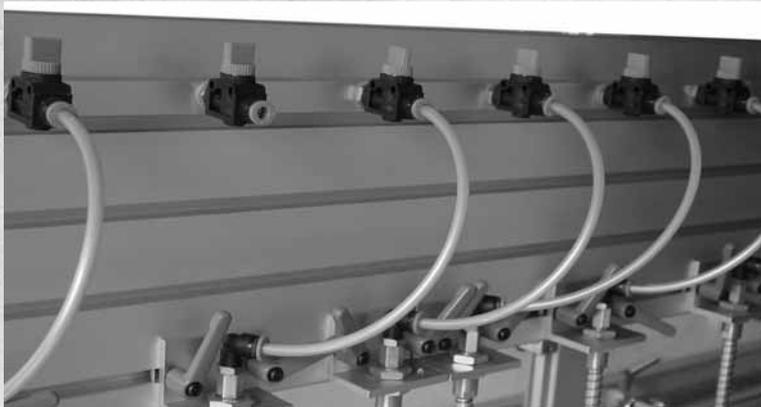
All standard pneumatic elements with thread G 1/8" und G 1/4" can be used with all standard MiniTec profiles. Fixing is possible at any desired point.
