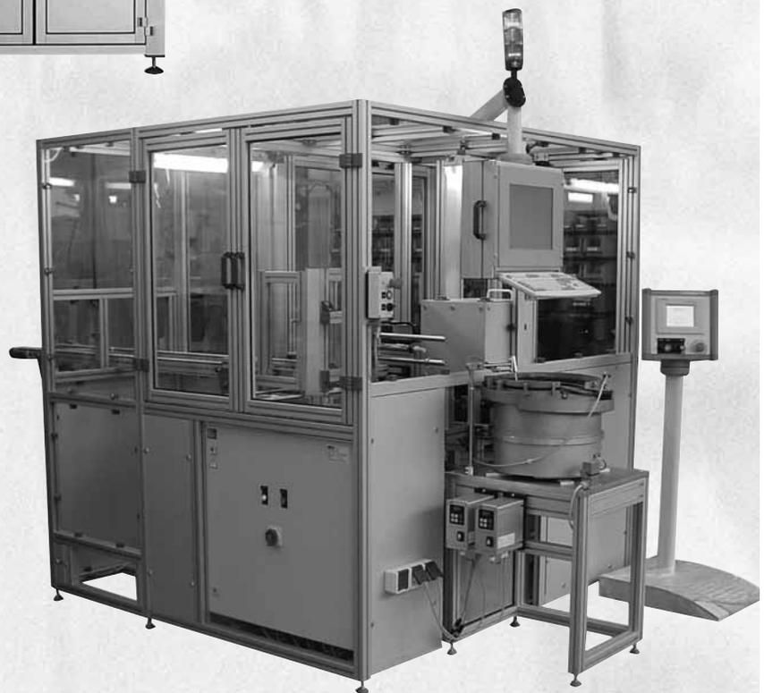
Measuring and surfacecheck of high-precision set screws for commonrail pumps
